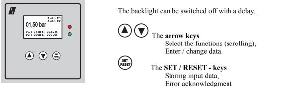
The red LED flashes when warning. The green LED flashes with inactive control The red LED will light up if a fault occurs. The green LED is lit when the control is active.
