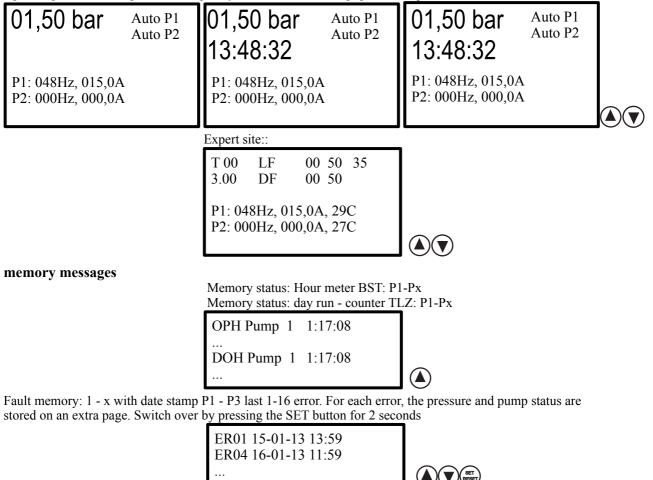
Between the displays operation can be changed with the arrow keys  $\blacktriangle$  and  $\triangledown$ .
