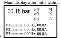
If the initialization goes wrong, there is an error message. With ER101 the frequency inverters cannot be reached. Check the Modbus connection / mains voltage of the frequency inverter.
